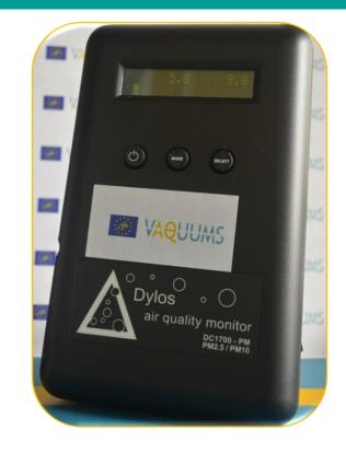
The Dylos DC1700 is a battery operated laser particle counter with 2 size ranges (>0.5 & >2.5 microns). In addition it can also display mass concentrations (PM2.5 and PM10). It is suitable for indoor and outdoor air quality monitoring. It has multiple modes including minute, hour and day.
